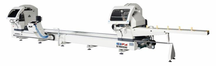
3 axis servo controlled double head cutting machine with 600 mm saw blades GEMINI – VI is ideal for cutting aluminum and PVC profiles in various angles and thickness. GEMINI – VI is designed for cutting larger profiles.
